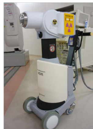
Figure 3. Brachytherapy therapy machine using radioactive iridium source
