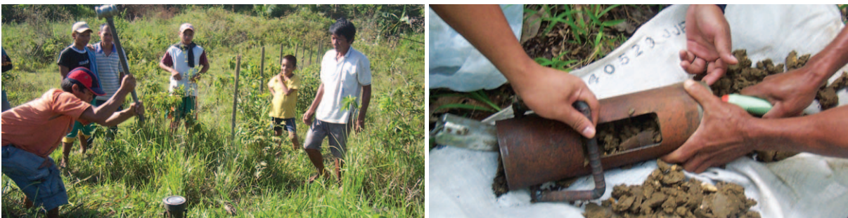
Figure 8: Collection of bulk soil samples for assessing soil erosion and sedimentation rates under different land uses in the Philippines using Fallout Radionuclide (FRN) analysis
