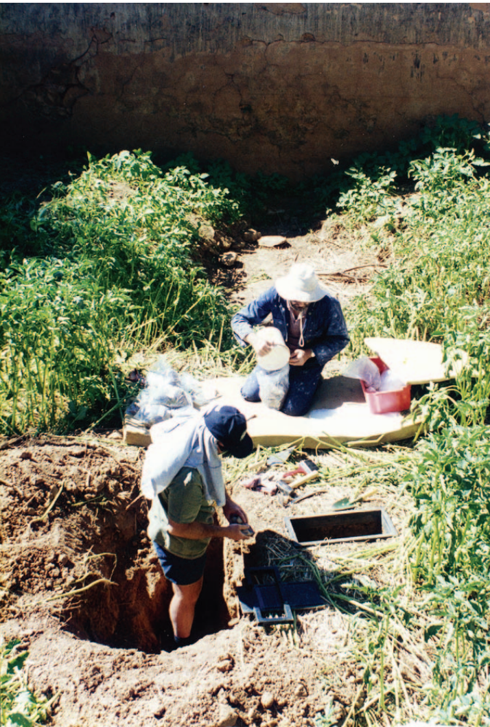
Figure 4: Collection of samples for the assessment of reservoir sedimentation rates in an arid environment in South East Australia using fallout radionuclide techniques
