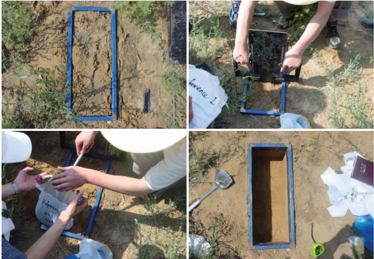
Figure 9: Use of scraper plates in Chinese Loess Plateau for detailed soil sampling before FRN analysis
