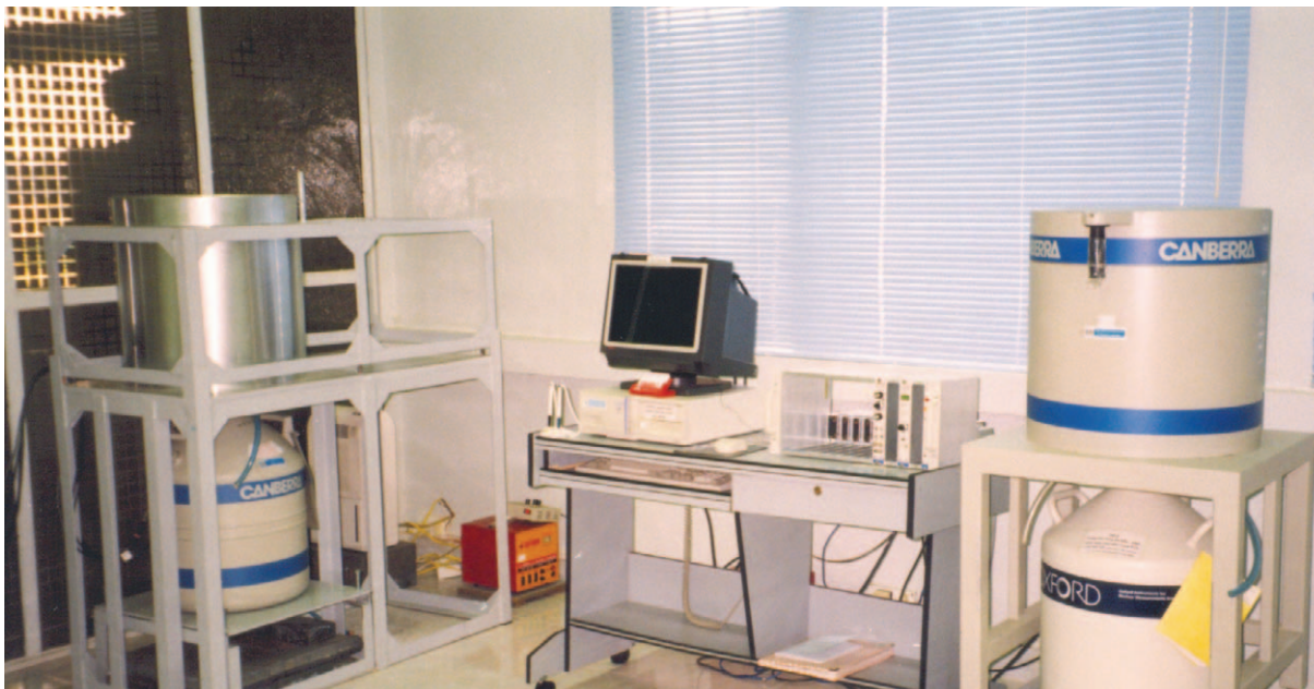
Figure 11: Analysis of samples for FRN analysis by using high purity germanium detectors with a 30% relative efficiency in Vietnam
